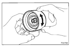
(b) Check that the idler pulley turns smoothly. If necessary, replace the idler pulley.
