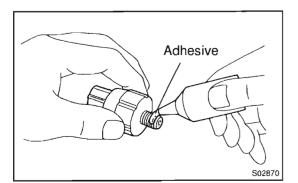
(f) Apply adhesive to 2 or 3 threads of the oil pressure switch. Adhesive:
