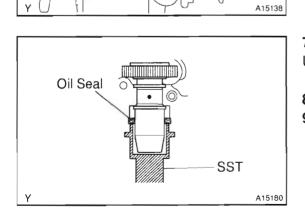
7. INSTALL CAMSHAFT OIL SEAL
