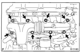
5. INSTALL TURBOCHARGER AND EXHAUST MAN-IFOLD ASSEMBLY
