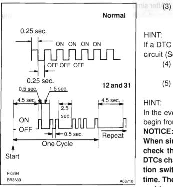
Read the DTC from the check engine warning light. As an example, the blinking patterns for codes; normal, 12 and 31 are as shown in the illustration.
