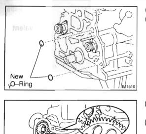
(d) Install 2 new O-rings to the cylinder block.(e) Install the timing gear case.
