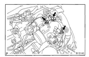
(d) Remove the 2 nuts, bolt, bracket, diesel throttle body and gasket.
