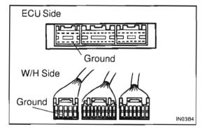
Measure the resistance between the ECU ground terminal and the body ground.
