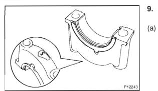
PLACE MAIN BEARING CAP AND LOWER THRUST WASHERS ON CYLINDER BLOCK
