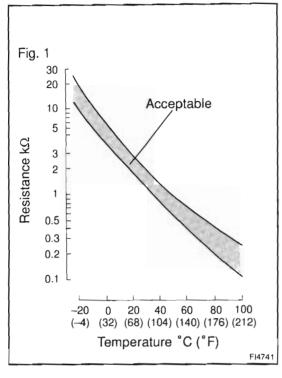
The fuel temperature sensor senses the fuel temperature. A thermistor built into the sensor changes the resistance value according to the fuel temperature. The lower the fuel temperature, the greater the thermistor resistance value, and the higher the fuel temperature, the lower the thermistor resistance value (See Fig. 1).
