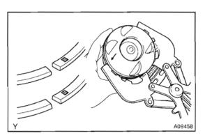
Using a piston ring expander, install the 2 compression rings with the code mark facing upward.
