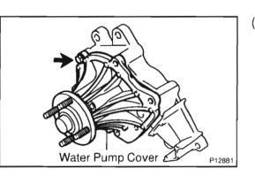
(b) Remove the bolt, water pump cover and gasket.
