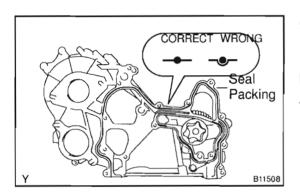
(b) Apply seal packing to the timing gear case as shown in the illustration.
