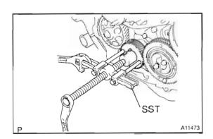
Using SST, remove the crankshaft timing gear.
