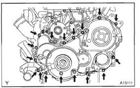
(c) Apply seal packing to the timing gear cover as shown in the illustration.
