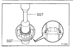
(b) Using SST and a press, press in a new bearing. SST 09214–76011, 09223–00010
