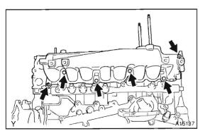
14. REMOVE INTAKE MANIFOLD
