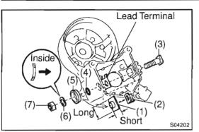
(e) Install new terminal C kit parts.
