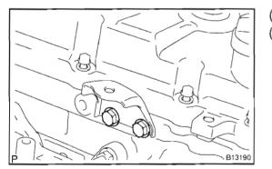
(e) Remove the 2 bolts and intercooler support bracket.(f) Remove the 4 clips and cover from the intercooler.
