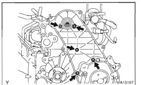
(b) Apply seal packing to the timing gear cover as shown in the illustration.
