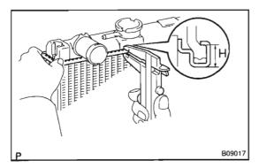
(b) Check the lock plate height (H) after completing the caluking.
