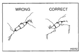
(2) To disconnect vacuum hoses, pull off the end, not the middle of the hose.
