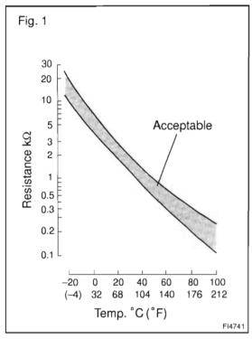
The atmospheric temperature sensor is built into the air flow meter and senses the atmospheric temperature. A thermistor built in the sensor changes the resistance value according to the atmospheric temperature. The lower the atmospheric temperature, the greater the thermistor resistance value, and the higher the atmospheric temperature, the lower the thermistor resistance value (See Fig. 1).
