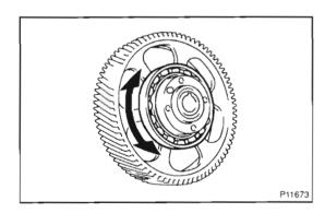
2. INSPECT RADIAL BALL BEARING BEARING
