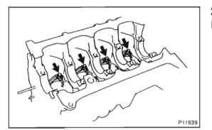
Remove the 4 check valves and oil nozzles.
