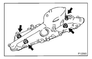
8. SEPARATE OIL COOLER AND OIL COOLER COVER Remove the 4 nuts, oil cooler and 2 gaskets from the oil cooler cover.
