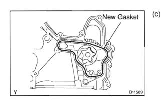
Place a new gasket into the groove of the timing gear case as shown in the illustration.
