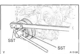
Using SST, install and torque the plate bolt.
