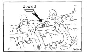
(k) Set the washer on the nozzle holder clamp as shown in the illustration.
