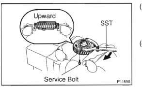
(e) Using snap ring pliers, install the snap ring.
