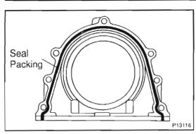
(b) Apply seal packing to the retainer as shown in the illustration.
