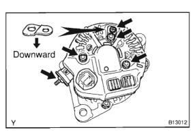
(b) Install the end cover and plate terminal with the bolt and 3 nuts.
