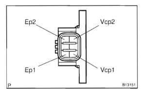
(b) Using an ohmmeter, measure the resistance between each terminals.
