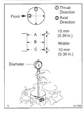
Using a cylinder gauge, measure the cylinder bore diameter at positions A, B and C in the thrust and axial directions. **Standard diameter:**
