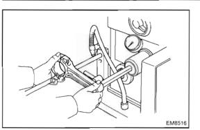
(f) Using a pin hole grinder, hone the bushing to obtain the standard specified clearance (See page EM–72) between the bushing and piston pin.
