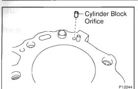
**4. INSTALL CYLINDER BLOCK ORIFICE** Install the cylinder block orifice to the cylinder brock.
