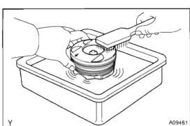
(c) Using solvent and a brush, thoroughly clean the piston. **NOTICE:**
