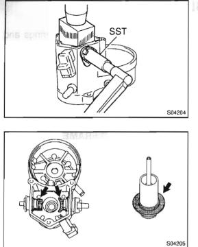
SST 09810–38140 Using SST, tighten the nuts to the specified torque.
