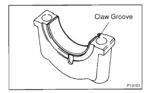
(b) Align the bearing claw with the claw groove of the main bearing cap, and push in the 5 lower bearings.
