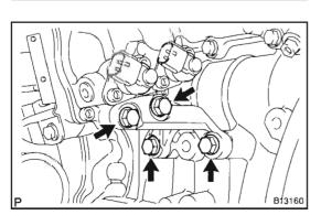
(e) Connect the 3 fuel hoses to the supply pump.
