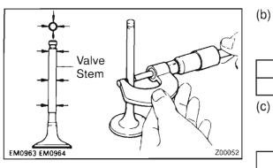
(b) Using a micrometer, measure the diameter of the valve stem.
