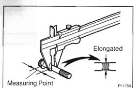
Using vernier calipers, measure the minimum diameter of the compressed bolt at the measuring point.
