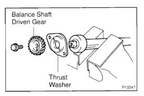
(b) Remove the bolt, balance shaft driven gear and thrust washer.
