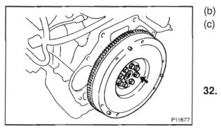
(b) Install the flywheel or drive plate on the crankshaft.
