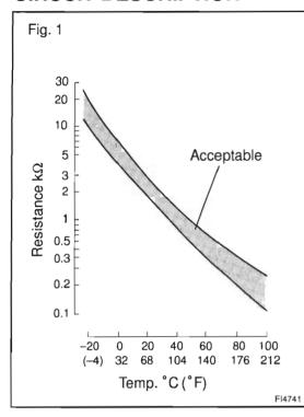
The intake air temperature sensor is built into the intake manifold and senses the intake air temperature. A thermistor built in the sensor changes the resistance value according to the intake air temperature. The lower the intake air temperature, the greater the thermistor resistance value, and the higher the intake air temperature, the lower the thermistor resistance value (See Fig. 1).
