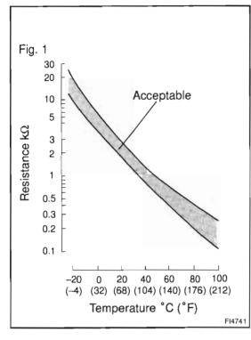
The water temperature sensor senses the coolant temperature. A thermistor built into the sensor changes the resistance value according to the coolant temperature. The lower the coolant temperature, the greater the thermistor resistance value, and the higher the coolant temperature, the lower the thermistor resistance value (See Fig. 1).
