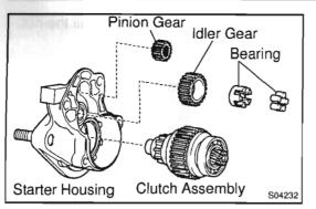
(c) Place the starter housing, pinion gear, bearing, idler gear and clutch assembly on the starter housing.
