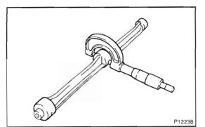
(b) Using a micrometer, measure the diameter of the balance shaft main journals.
