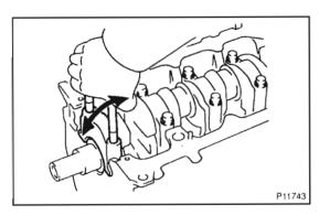
(b) Using the removed main bearing cap bolts, pry the main bearing cap back and forth, and remove the main bearing caps, lower bearings and lower thrust washers (No.5 main bearing cap only).
