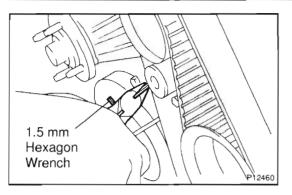
(c) Remove the 1.5 mm hexagon wrench from the tensioner.
