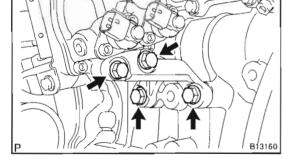
Remove the 4 bolts and supply pump stay. **REMOVE SUPPLY PUMP**
