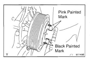
(a) Install the pump pulley, the fluid, fan and coupling assembly with the 4 nuts.
