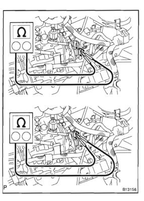
(b) Using an ohmmeter, measure the resistance between terminals as shown.
