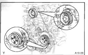
5. SET NO.1 CYLINDER TO TDC / COMPRESSION Set the timing pulley at each position.
