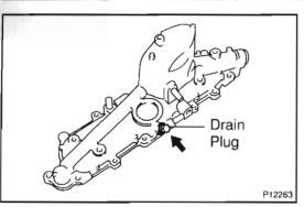
**INSTALLATION** 1. INSTALL ENGINE DRAIN PLUG
