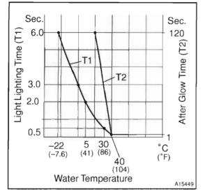
When the ignition switch turns ON, the engine ECU calculates the glow indicator lighting time/heating corresponding to the coolant temperature at that time and turns ON the glow indicator light/glow plug relay.
