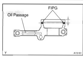
(f) Apply seal packing to the camshaft bearing cap No. 1 as shown in the illustration.
