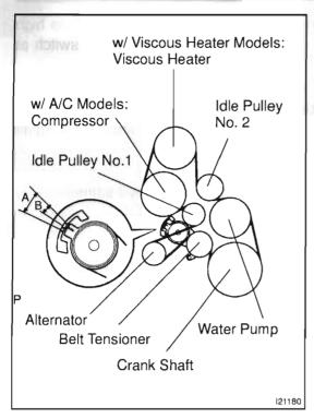
6. **INSPECT DRIVE BELT TENSION** Check that the tension is within A range on the auto tensioner
