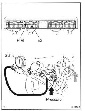
(f) Using SST (turbocharger pressure gauge), apply pressure to the turbo pressure sensor in 19.6 kPa (0.20 kgf/cm<sup>2</sup>, 2.84 psi) segments to 98.0 kPa (1.00 kgf/cm<sup>2</sup>, 14.2 psi).
