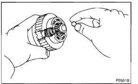
(c) Using a screwdriver, hold the brush spring back, and connect the brush into the brush holder. Contact the 4 brushes.
