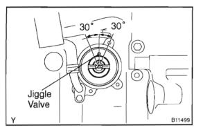
(b) Install the thermostat with the jiggle valve upward. HINT:
