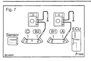
(2) Disconnect connector "B" and measure the resistance between terminal 1 of connector "A" and body ground, and terminal 1 of connector "B2" and body ground.
