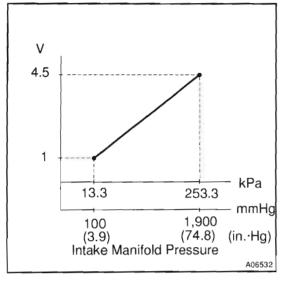
The turbo pressure sensor is connected to the intake manifold. The engine ECU detects the intake manifold pressure as a voltage by the sensor. The engine ECU uses the intake manifold pressure signal for correction of injection volume control and injection timing control.
