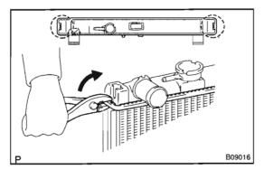
The points shown in the rib sides near here cannot be staked with SST. Use pliers similar object and be careful not to damage the core plates.
